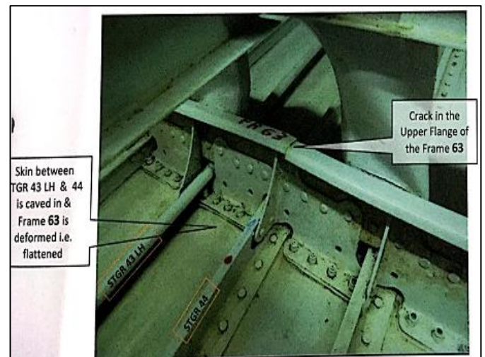
Aft frame No.63 cracked due tail strike
