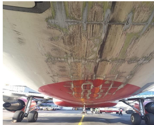
Damaged aircraft belly
