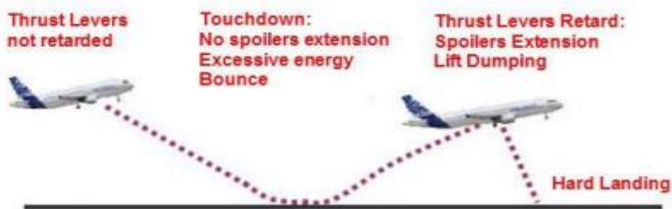
Aircraft fitted with older version SEC112 without Phase Lift Dump function
